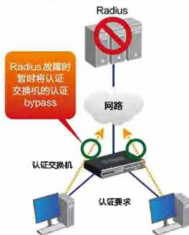
认证 bypass 机制 Radius 故障时暂时 bypass 认证
